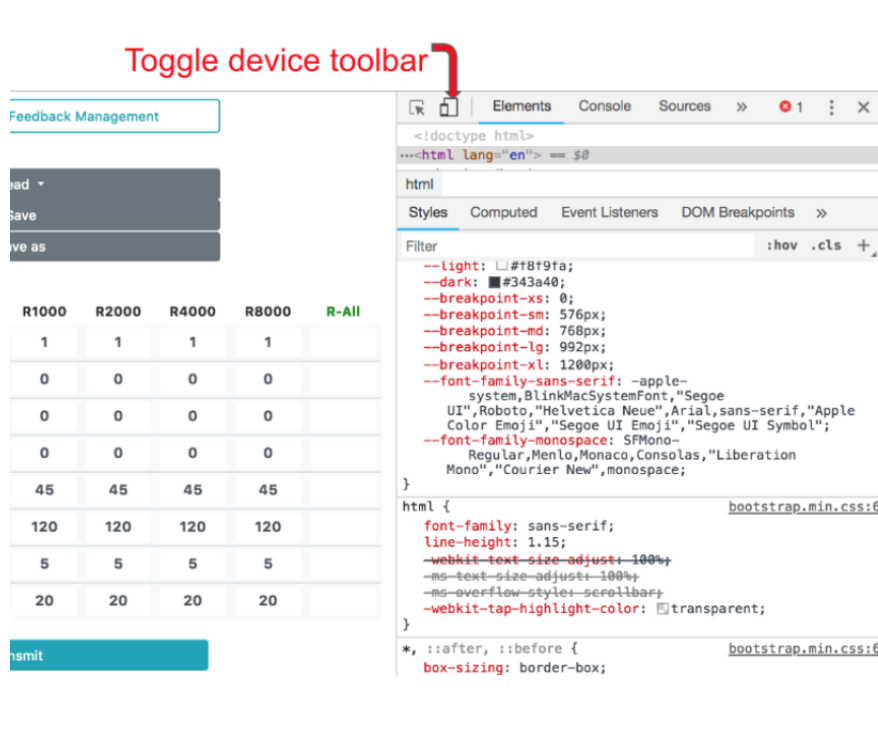
Figure 2.9: OSP Web Apps in Console Mode. If you are using a browser such as Chrome, you can right click in the browser window and choose Inspect. In this mode, you can view exchange of information between RT-MHA and the app. You can also change the app to be formatted for laptop and mobile devices using the Toggle Device Toolbar icon.
